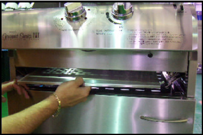
Figure 2. Place the plate under grill control panel and move plate towards the back. Slip the back edge of the vaporizer plate over the plate with the holes (see Figure #3). The grill need not be tipped to insert the plate. This figure for display purpose only.
