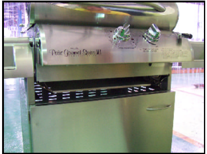
Figure 4. Vaporizer plate installed.
